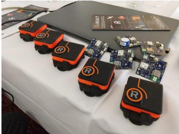
The project's wearable enhances the localisation of the personnel deployed on the ground. It also incorporates oxygen and motion sensors, to detect intoxication due to the lack of oxygen on the first-responders, as well as stumbles and falls.
